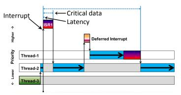
When the interrupt occurs the ISR is activated and will read the hardware registers. The ISR can't communicate with the RTOS so it will defer that operation. This architecture outperforms the unified architecture in latency and reads critical data faster. The RTOS will queue the data for the deferred operation so it has no negative impact on performance.
